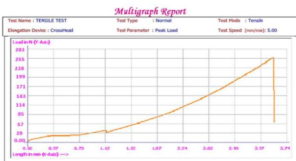
Figure 7: Multi-Graph Report of Tensile Test 5 % Weight Fraction.
