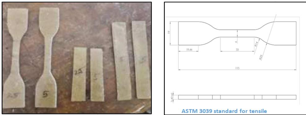
**Figure 4: Testing Specimens**
