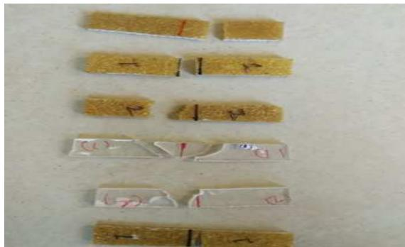
Figure 6: Tested Specimens of Flexural Test
