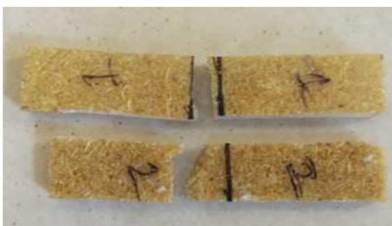
Figure 7: Tested Specimens after Impact Test.
